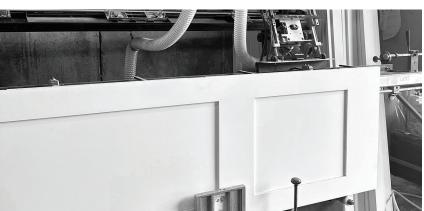
Norfield Magnum Prehung Door Machine: Interior, exterior, and commercial doors, almost infinite hinge patterns, 8-0 door and jamb ready, automated drilling and faceplate routing.
