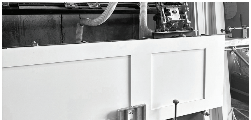
Norfield Magnum Prehung Door Machine: Interior, exterior, and commercial doors, almost infinite hinge patterns, 8-0 door and jamb ready, automated drilling and faceplate routing.
